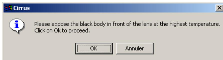
Place your high temperature reference in the measurement position (close to the lens, in an unfocused area) then click on "OK".
