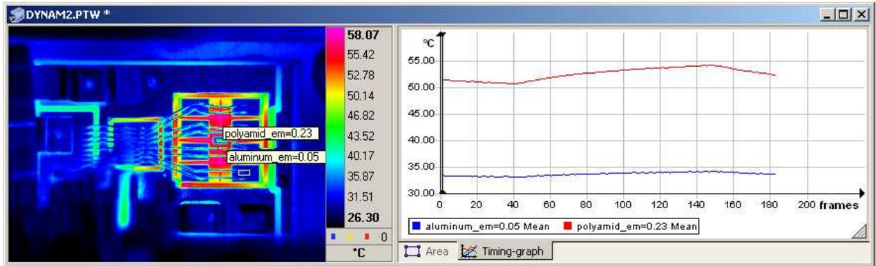
Thermal image after emissivity correction
