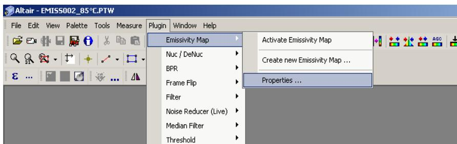
Select the map of emissivity file and select activate. The map is applied to the current thermal image
