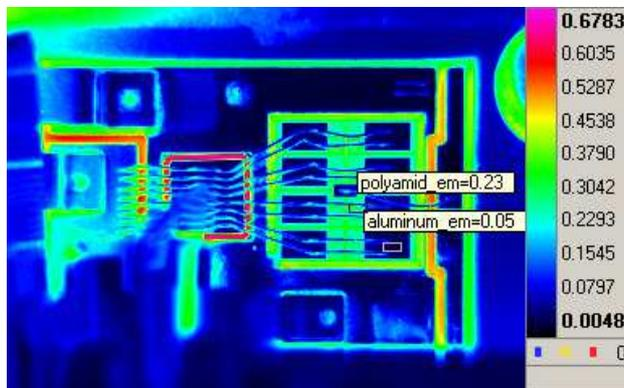
Thermal image before emissivity correction
