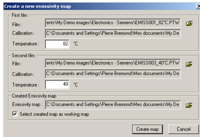
Give a name of the result file (map of emissivity) and launch the process to compute the emissivity map by the button “Create map”
