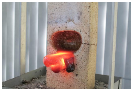
Figure 2. Photograph of the melting of refractory brick, showing the oval shape of the melted material.
