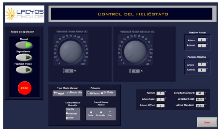
**Fig. 6. Main screen for manual mode.**
