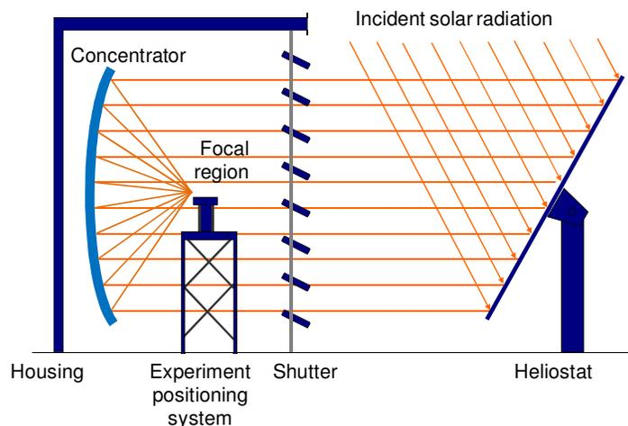
**Fig. 1. Schematic of the components of a solar furnace**
