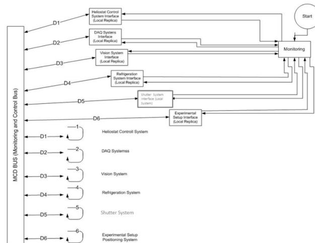
**Fig.11. Diagram of SCADA System for controlling the HRFSE.**
