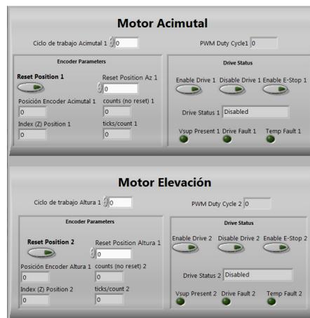
**Fig. 4. Front Panel of the basic program for motor movement**
