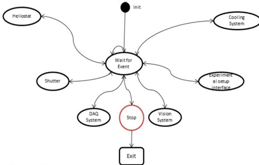
**Fig. 2. State machine diagram of the central control**
