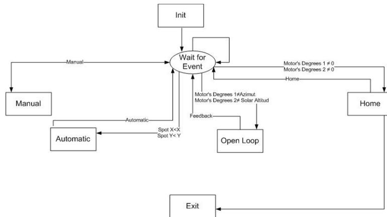
**Fig. 5. Diagram of the state machine for the heliostat control.**
