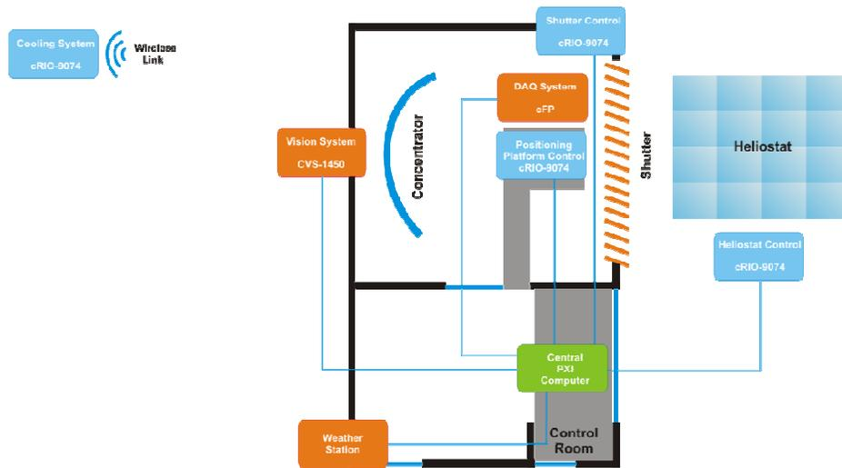
**Fig. 3. HRFSF control and data acquisition diagram**
