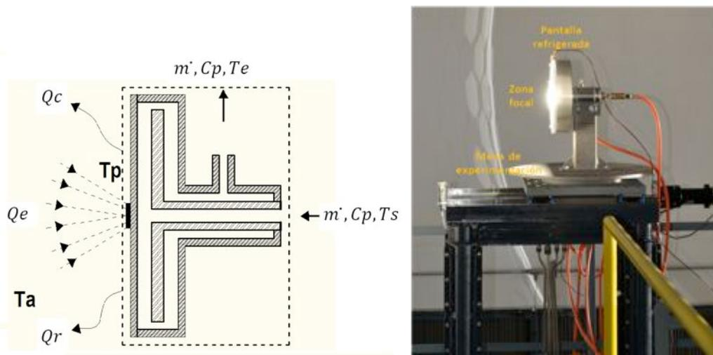
Fig. 3. Left: Cross section of the cooled flat plate target showing the energy balance. Right: Experimental set up with the cooled flat plate target at the focal zone of the HFSF.
