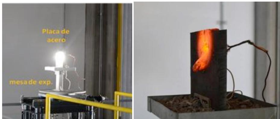
Fig. 5. Left: experimental set up of the carbon steel plate for the melting test. Right: picture of the melted plate.
