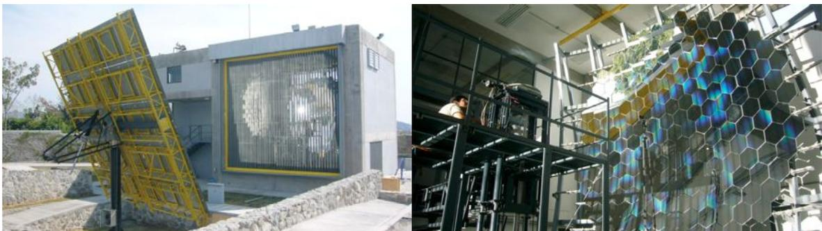
**Fig. 1. Left: Picture of the HRFSF showing heliostat, shutter and concentrator. Right: picture of the concentrator with its 211 facets.**
