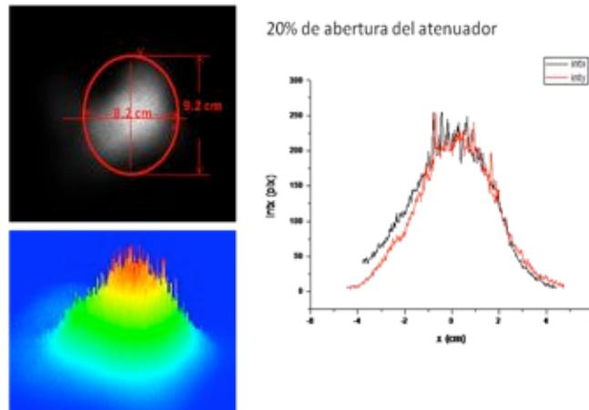
Fig. 4. Image taken with the CCD camera and the flux distribution profiles.
