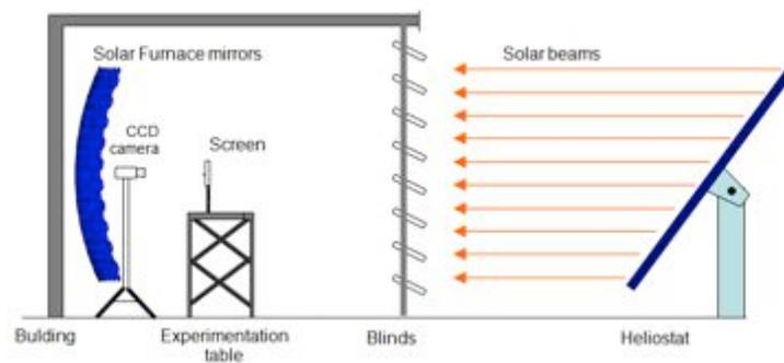
Fig. 2. Schematic arrangement of the experimental setup.
