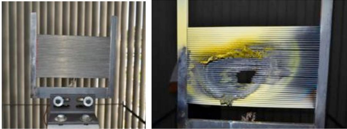
**Fig. 6. Left: experimental set up of the tungsten rods set. Right: picture of the melted rods.**
