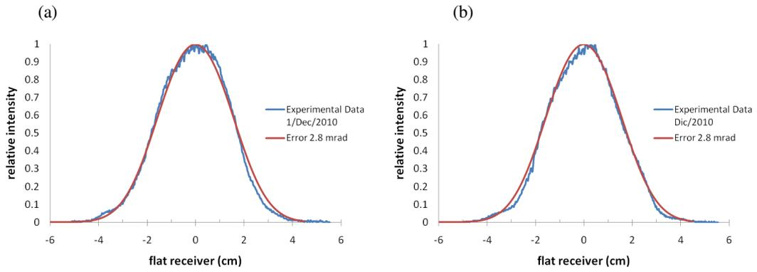
**Fig. 5. Comparison of experimental and theoretical irradiance profiles for image 1 taken with the heliostat 36 m<sup>2</sup>. (A) Vertical profile. (b) Horizontal profile**
