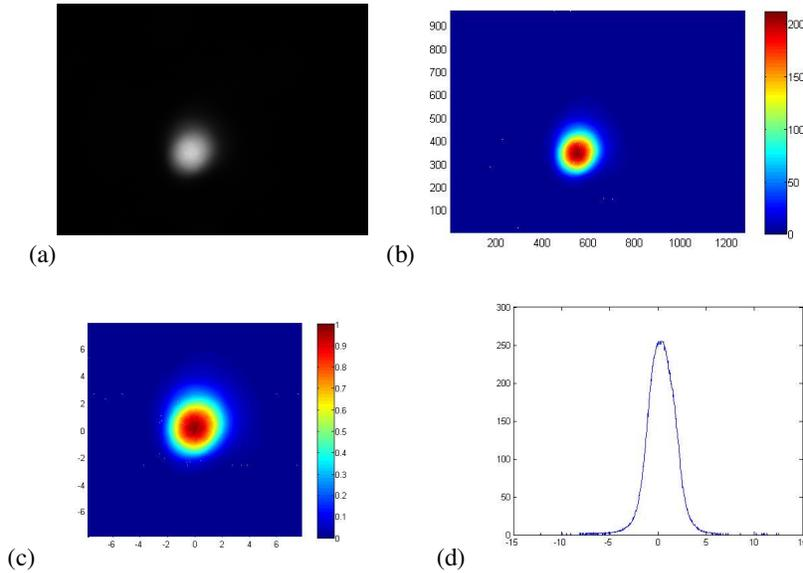
**Fig. 4. (a) CCD picture from spot at the receiver at the focal point. (b) Picture translated to the computer for processing. (c) Image centered and processed. (d) Irradiance profile from the solar spot**
