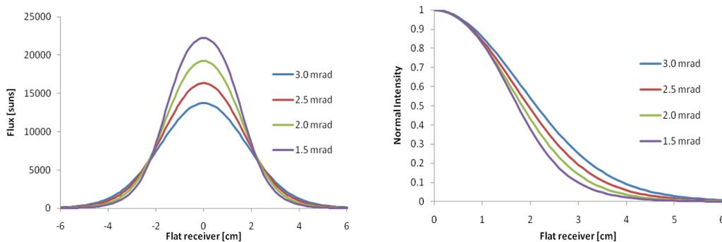
**Fig. 8. Irradiance profiles from HSAFR. (a) Absolute, (b) Relative**
