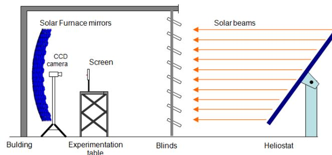
**Fig. 3. Schematic arrangement of the experimental setup**
