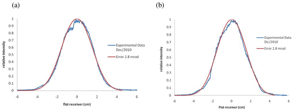
**Fig. 6. Comparison of experimental and theoretical irradiance profiles for image 2 taken with the heliostat 36 m<sup>2</sup>. (A) Vertical profile. (b) Horizontal profile**
