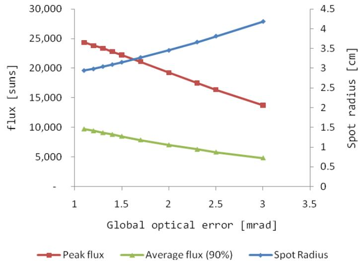
**Fig. 9. Variation of theoretical peak flux, average flux and spot radius against optical error**
